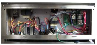
Control panel frame with computer removed.
